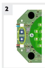
Identify the control board in the base of the beacon gallery and locate the array adjustment controls. There are two controls, each offering 8 levels of adjustment to the front and back projection. Note the white arrays projection. Note the white arrows printed on the board indicate which side of the beacon will be adjusted by
