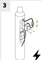
Move to the base compartment of the host post and fix the beacon transformer onto the column board using the four screw provided.
