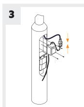
Move to the base compartment and fix the beacon transformer onto the column board using the 4 screws provided.
